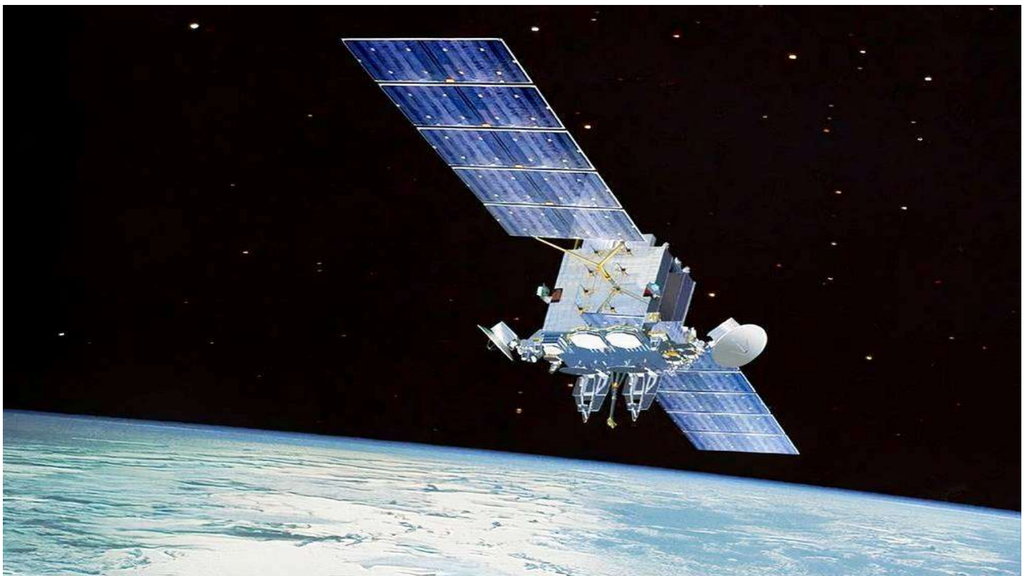
The Advanced Extremely High Frequency, or AEHF, system is a joint service satellite communications system that provides survivable, global, secure, protected and jam-resistant communications for high-priority military ground, sea and air assets. U.S. Air Force photo (DVIDS).
